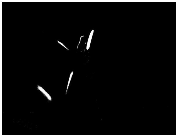
Figure 11 - Thresholded bottom view image after background subtraction
