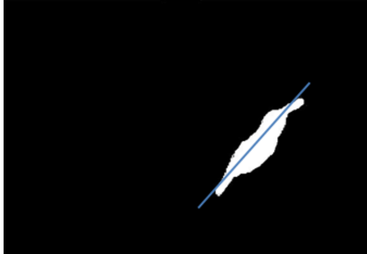
Figure 20 - Remaining body treated as single blob. 1st order ellipse fitted to blob, and angle measured.
