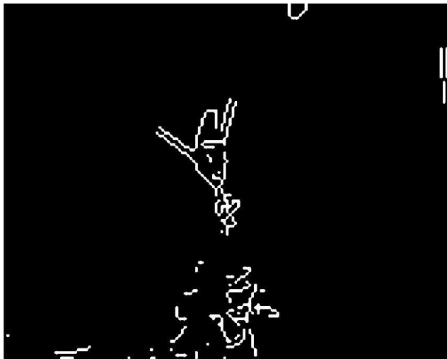
Figure 13 - Prewitt edge detection of raw bottom image
