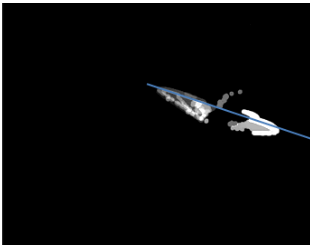
Figure 17 - Edge detected image used to remove extraneous blobs. Remaining blobs tracked and a line fitted to centroids to determine stroke plane angle.
