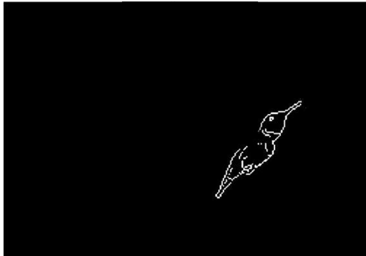
Figure 19 - Stationary objects subtracted from edge detected image.
