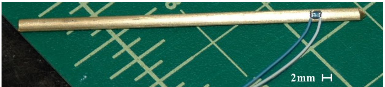
Figure 11- 600 series surface mount RTD epoxied to heater pin and soldered to leads.
